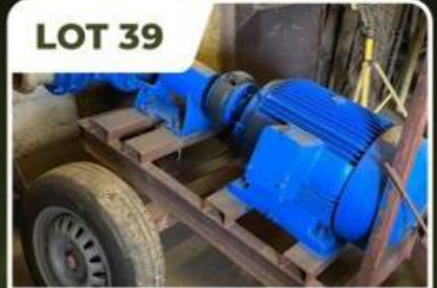
Siemens 37kw Electrical Motor + Normaflo NF 65-250 Pump on Chassis
