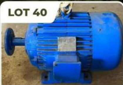
22kw Electric Motor 2900 RPM 3-phase
